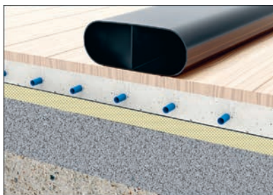
Shallow duct on top of the floor covering
